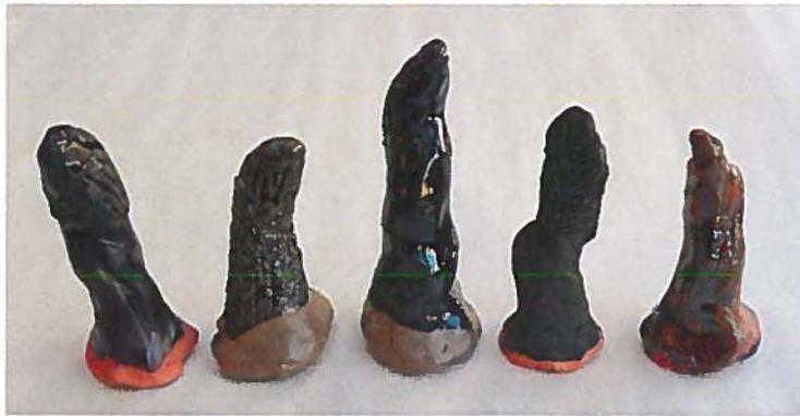
Fig. 1. Left to right: Mayco Foundations Black Velvet Matte Cone 05, Licorice Black Cone 5, Black Gloss Cone 5, Black Velvet Underglaze Cone 05, and Copper Carbonate/ Gerstley Borate Stain Cone 05.
