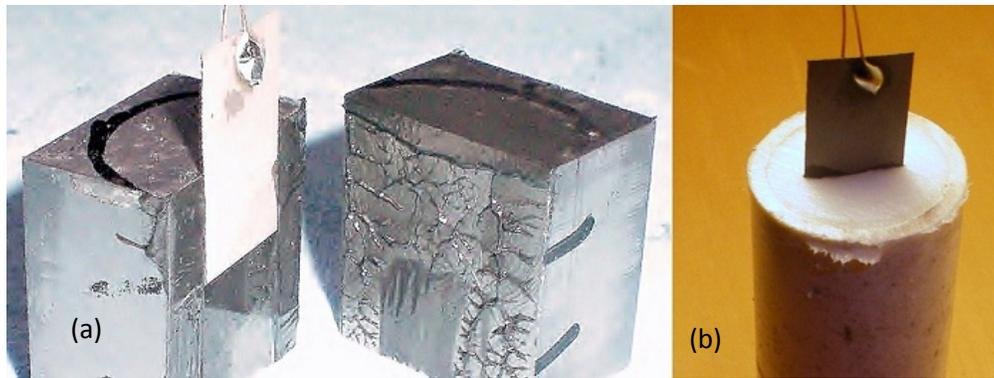
*Figure 8.* - Two methods to form the anchoring medium, casting blocks (a) and lard surface (b). Epoxy is poured into a housing that rests upon either of these horizontal surfaces. Care is taken to ensure a level casting surface that resists bonding with the anchoring medium. Any type of housing may be used in conjunction with the casting surface. Consistency in housing dimensions is recommended.
